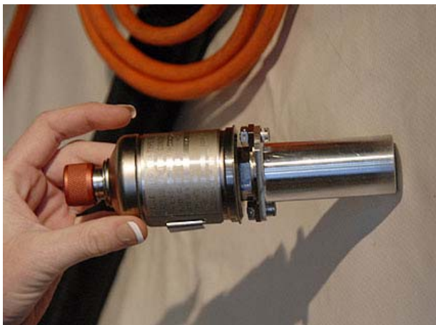
A technician holds one of Discovery's gaseous hydrogen flow control valves after its removal. The valves channel gaseous hydrogen from the main engines to the external tank.
